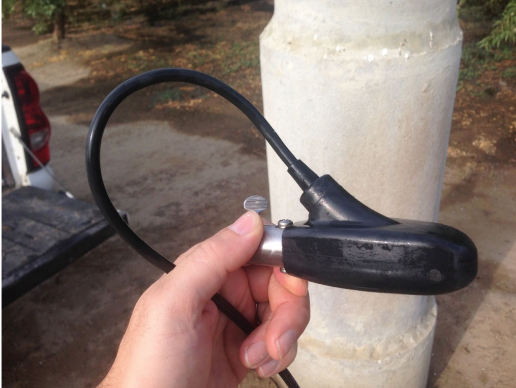
Figure F5.7. Hach FH950 Magnetic Velocimeter with Measurement Access Vent Pipe in the Background.
