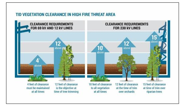
All State Responsibility Area requirements are incorporated into TID's Fire Zone Standard. SRA requirements are contained in Section 4292 and 4293 of the California Public Resource Code. Exemptions to the conductor clearance requirements are contained in Sections 4292, 4294, and 4296 of the California Public Resource Code. Exemptions are found in Title 14, Section 1257, of the California Code of Regulations. TID also references the Power Line Fire Prevention Field Guide published by Cal Fire.
