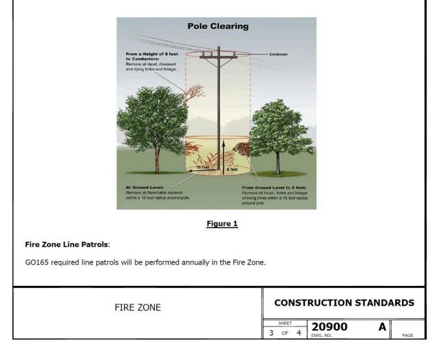
Figure 11: Excerpt from TID Fire Zone Standard
